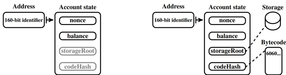
Figure 2.2: State of an EOA on the left and of a contract-account with EVM bytecode storage for contract-data on the right [5].
